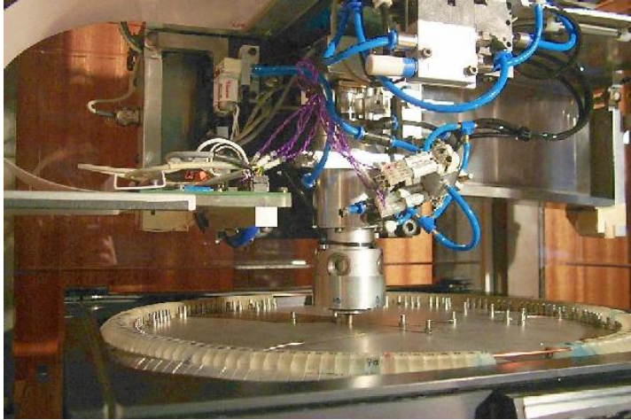
The 6df Interchangeable Field Plate This plate features 150 retractable fibers, controlled via software to take measurements. Credit: The RAVE Collaboration
