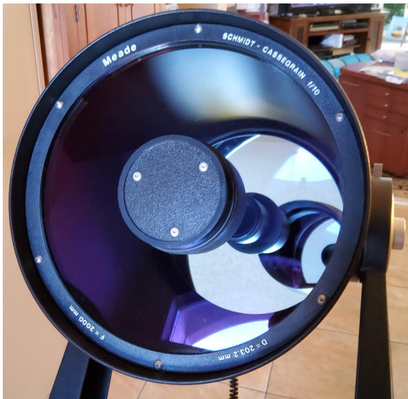
The business end of a Meade 2080 Schmidt-Cassegrain Telescope
