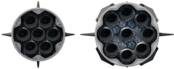
Comparison of engine layout between current New Glenn booster and 9x4. Blue Origin image.
